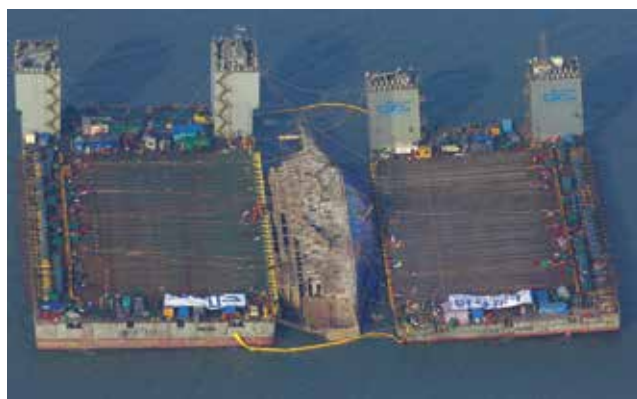
The damaged ferry between two barges after being raised
